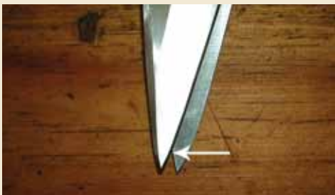
Photo 1 shows how much the blades are cutting into each other. Photo 2 after setting the shears
