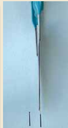
Photo 1 shows how much the blades are cutting into each other. Photo 2 after setting the shears
